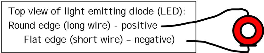
Figure 1: LED Schematic
