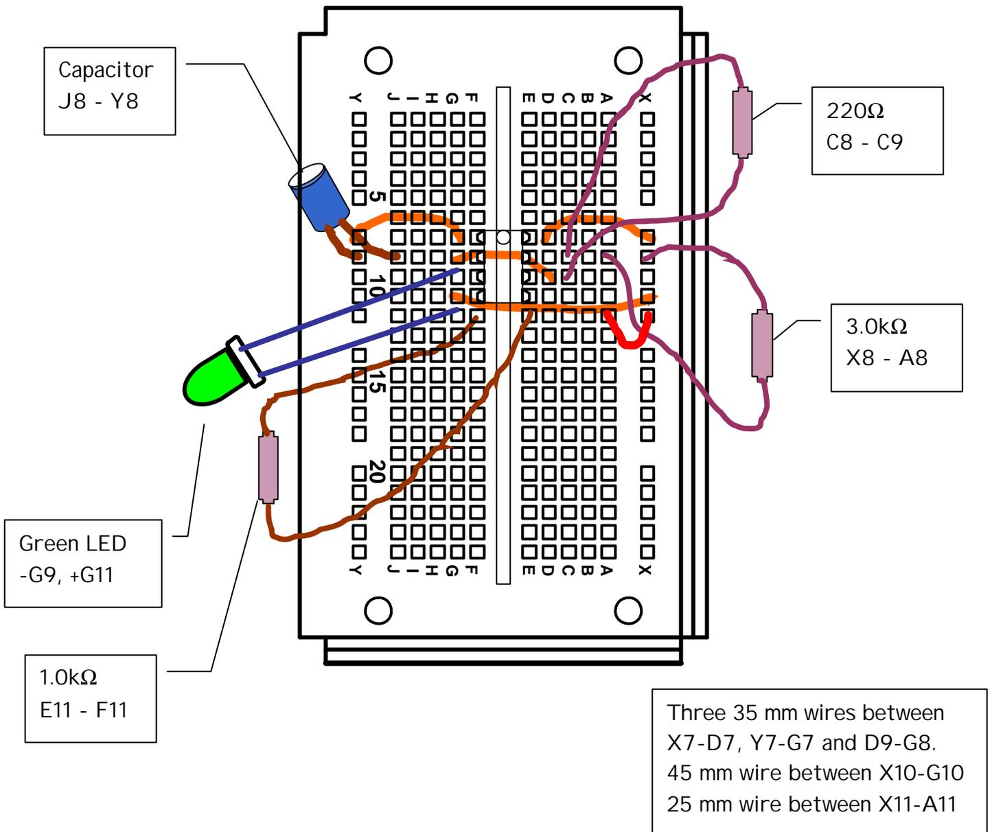
Figure 4: Schematic Diagram for Power Saving Beacon (G)
