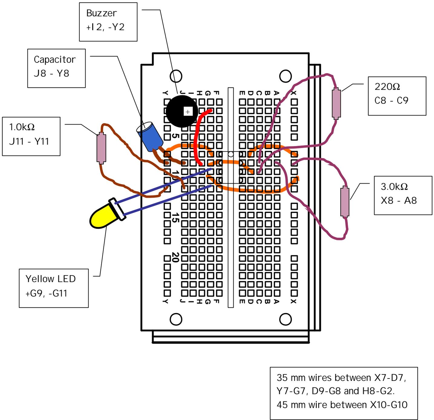
Figure 3: Schematic Diagram for Deluxe Beacon (Y)
