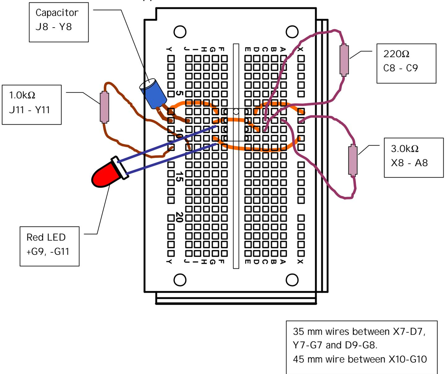
Figure 3: Schematic Diagram for Plain Beacon (R)
